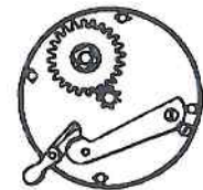
10. Snyder Reel Gearing.
