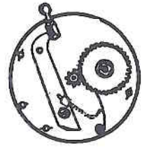
12. Massie's Reel Gearing.
