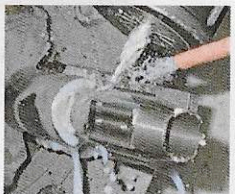
3 foot fittings cutted out in a time from a bar-stock SUS.
