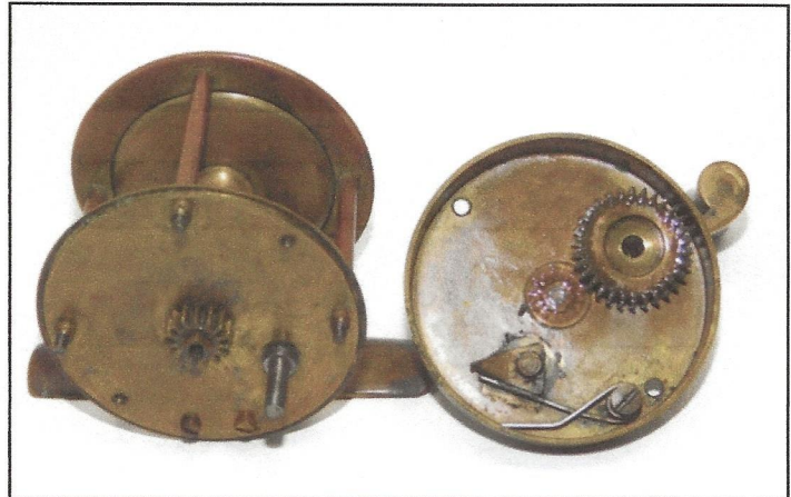
Photos showing a Malleeson marked reel. A unique feature seen on the reel is the click mechanism. Malleeson favored a rotating mechanism to engage the click rather than a sliding one as seen on other reels made at this time. A quarter turn of the little knob on the front plate rotates the triangular dog. The dog is held in place by a spring loaded wire.
