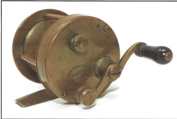
Photos showing a Malleeson marked reel. A unique feature seen on the reel is the click mechanism. Malleeson favored a rotating mechanism to engage the click rather than a sliding one as seen on other reels made at this time. A quarter turn of the little knob on the front plate rotates the triangular dog. The dog is held in place by a spring loaded wire.
